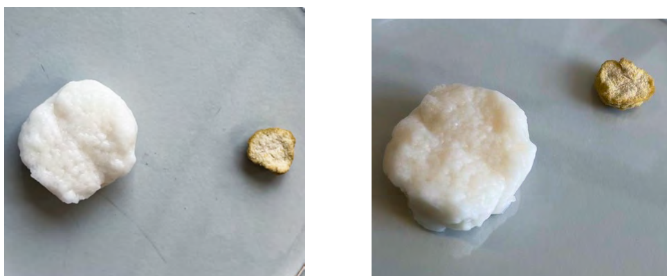
Figure 3.10: Optical images of a wet BMBC sample (left) next to a dried zein-coated BMBC sample (right). The left image depicts the samples from above, while the right image is a high-angle shot of the samples. The zein-coated sample was prepared according to the third protocol, as described in Section 2.3.
